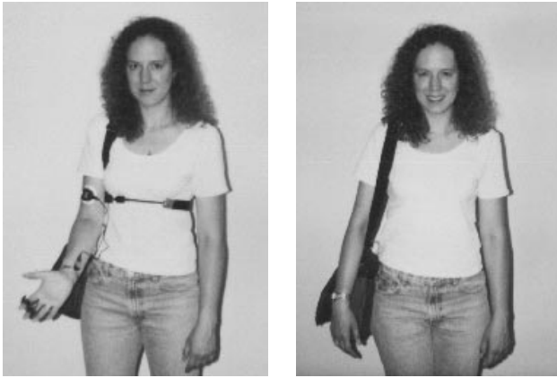
Figure 4: Shown left, the physiological sensors for the affective wearable, a respiration sensor, worn around the chest, an EMG, shown here on the bicep, a BVP attached to the wrist and a GSR sensor shown worn on two fingers. Shown right, the same sensors under clothing become unobtrusive. In this photo the respiration sensor is in the same location, EMG is on the trapezius muscle (shoulder), and BVP and GSR sensors are on the back. The sensors are connected to a wearable computer with the PalmPilot interface, worn in the satchel on the left shoulder. Photo courtesy of Justin Seger.
