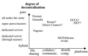
Figure 14: Examples of Levels of Decentralization in Various P2P Systems.
