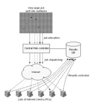
Figure 15: Distributed computing over the Web
