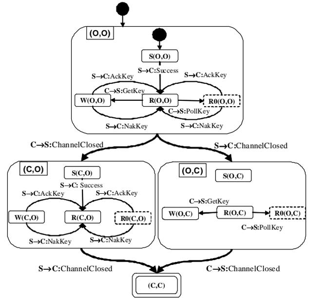
Figure 4: KeyboardDeviceContract with the Implicit States for Channel Closing shown as a Hierarchical State Machine
