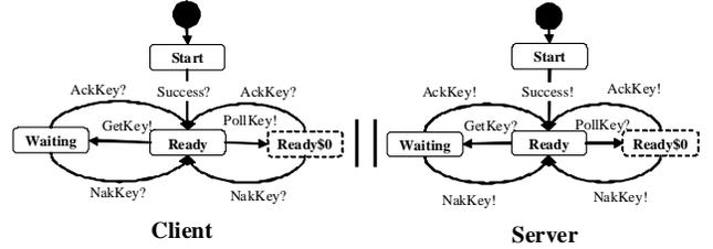
**Figure 7: Projection of the KeyboardDeviceContract to the Client and the Server**
