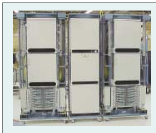
Figure 11. Lucent LambdaRouter optical cross-connect system. The system is fully NEBS level 3 compliant and is beginning large-scale commercial deployment.
