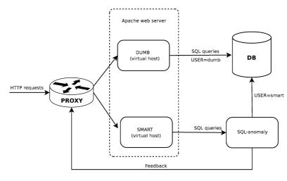
Fig. 6. Testbed architecture.
