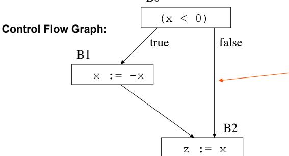
Test set {x=-1} does not execute this edge, hence, it does not give branch coverage
