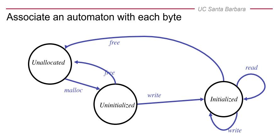
Missing transition edges indicate an error
