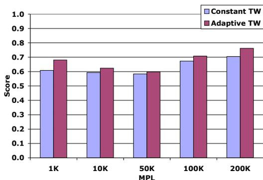
Figure 8: Average of best scores across all benchmarks, models, and analyzers for the Constant and Adaptive TW policies using the anchoring policy for detecting the beginning of a phase.
