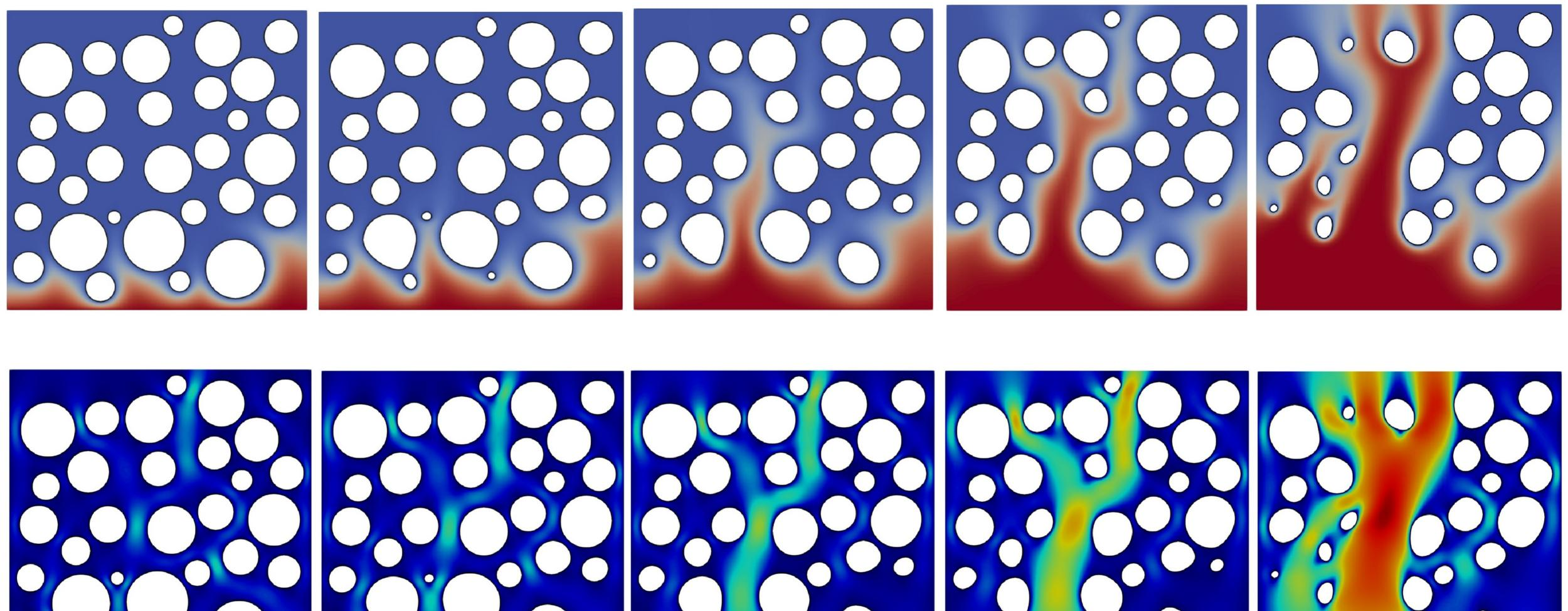
Left to right: time evolution of solute concentration (top) and fluid velocity (bottom) in an evolving porous medium, e.g. due to dissolution
