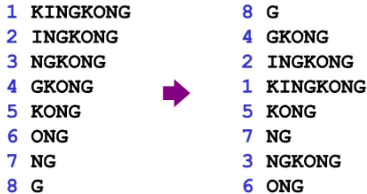
Figure 3.1: Suffix array built on the string “KINGKONG”. On the right all the suffixes of the word are sorted lexicographically. S[i] contains the original position in the text of the i – th suffix considered in lexicographic order.
