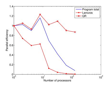
Figure 16: Parallel efficiency of individual program components on different numbers of processors for the problem size of N = 1564.
