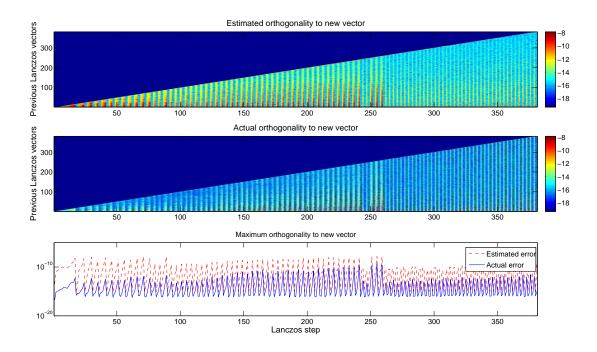
Figure 8: Loss of orthogonality, both actual and estimated, vs. Lanczos step for  $\eta = 0$ , or full reorthogonalization (not after every Lanczos step though). The base 10 log of the magnitude of the orthogonality is shown in the colormaps. Reorthogonalizations are visible as vertical blue streaks in the colormaps.
