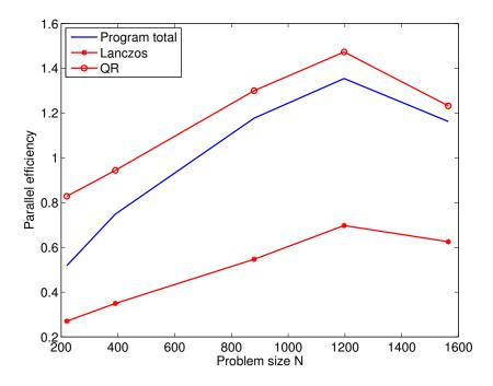
Figure 14: Parallel efficiency of individual program components on 8 processors for different problem sizes.
