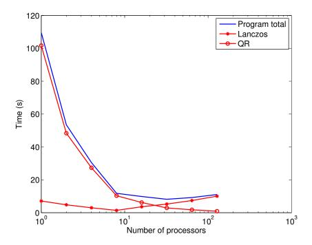
Figure 15: Time individual program components took to run on different numbers of processors for the problem size of N = 1564.
