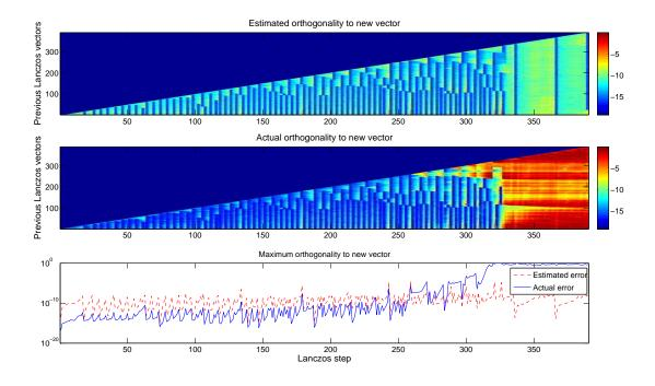
Figure 6: Loss of orthogonality, both actual and estimated, vs. Lanczos step for  $\eta = \epsilon^{0.80}$ . The base 10 log of the magnitude of the orthogonality is shown in the colormaps. Reorthogonalizations are visible as vertical blue streaks in the colormaps.
