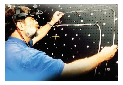
**Figure 1.3** Researchers at Boing used a see-through HMD to guide the assembly of wire bundles for aircraft. Courtesy of David Mizell.
