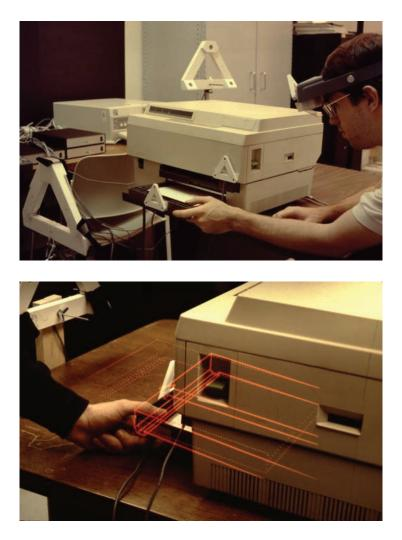
**Figure 1.4** (top) KARMA was the first knowledge-driven AR application. (bottom) A user with an HMD could see instructions on printer maintenance. Courtesy of Steve Feiner, Blair MacIntyre, and Doreé Seligmann, Columbia University.
