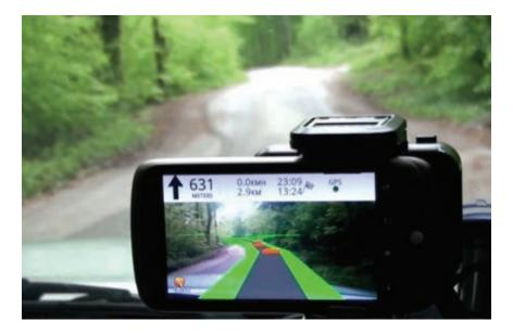
**Figure 1.22** Wikitude Drive superimposes a perspective view of the road ahead. Courtesy of Wikitude GmbH.
