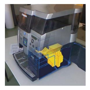
**Figure 1.16** Ghost visualization revealing the interior of a coffee machine to guide end-user maintenance. Courtesy of Peter Mohr.
