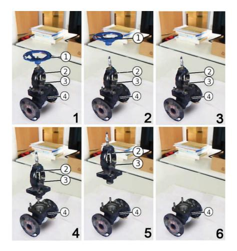
Figure 1.17 Automatically generated disassembly sequence of a valve. Courtesy of Peter Mohr.
