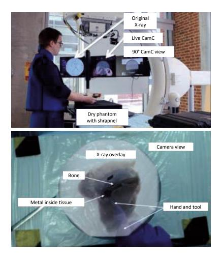
**Figure 1.19** The CamC is a mobile C-arm, which allows a physician to seamlessly blend between a conventional camera view and X-ray images. Courtesy of Nassir Navab.
