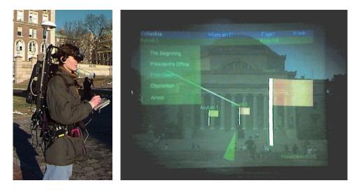
**Figure 1.8** The Touring Machine was the first outdoor AR system (left). Image of the *Situated Documentaries* AR campus tour guide running on a 1999 version of the Touring Machine (right). Courtesy of Columbia University.
