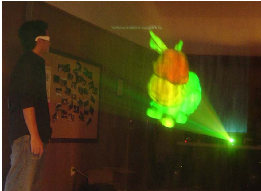
Figure 7: The pseudo-volumetric 3D FogScreen, displaying the Stanford Bunny [30] with ChromaDepth [25] stereoscopic imaging.
