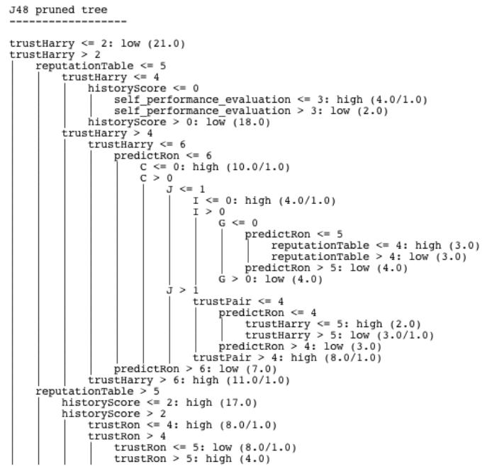
Fig. 6. Example of a J-48 Decision Tree learned from the survey (self-reported) assessments. The goal of the algorithm was to predict observed trust behavior in a hidden test set.
