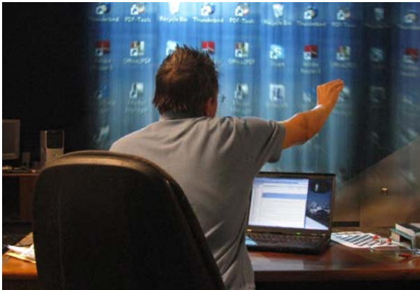
Fig. 2 The FogScreen could serve as a secondary display on a desktop environment, enabling a large virtual desktop, while being translucent and penetrable, thus being suitable for offices
