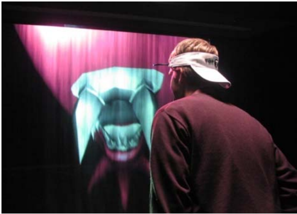
Fig. 12 The FogScreen can be used for freely accessible mid-air virtual reality spaces, here a 3D model of a cartoony shark, rendered from the perspective of a tracked user. The 3D shark appears fixed in space and the user can walk around it and even stick his head into the shark's mouth
