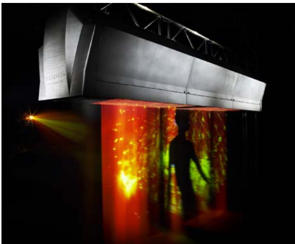
Fig. 5 The FogScreen creates a mid-air, walk-through image
