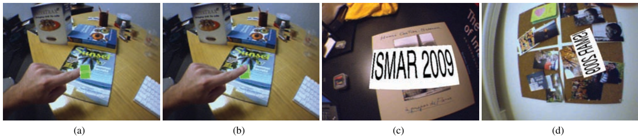
Figure 3: Occlusion detection and annotation. In a typical AR system, virtual objects like the synthetic green cube (a) are rendered on top of foreground objects, which breaks the AR illusion and hinders spatial comprehension. Using moving viewpoint background subtraction, we correct for occlusion artifacts (b). We also use the model for online text annotation (c), with accurate depth and normal information. A later frame from the same sequence (d) shows how the model expands to new areas as they are explored.
