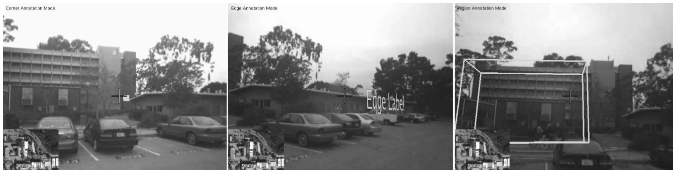
Figure 3: Example annotations as seen by the user in first person view mode. Left to right: (a) Corner annotations on the corners of two buildings are rendered as cubes. (b) An edge is annotated with a texture mapped onto the plane of the wall it denotes. (c) A region annotation is rendered as a wireframe bounding box. These renderings are not geared towards a particular application; rather, they are for illustrative purposes. Applications using these annotations would have visual representations tailored to their needs.
