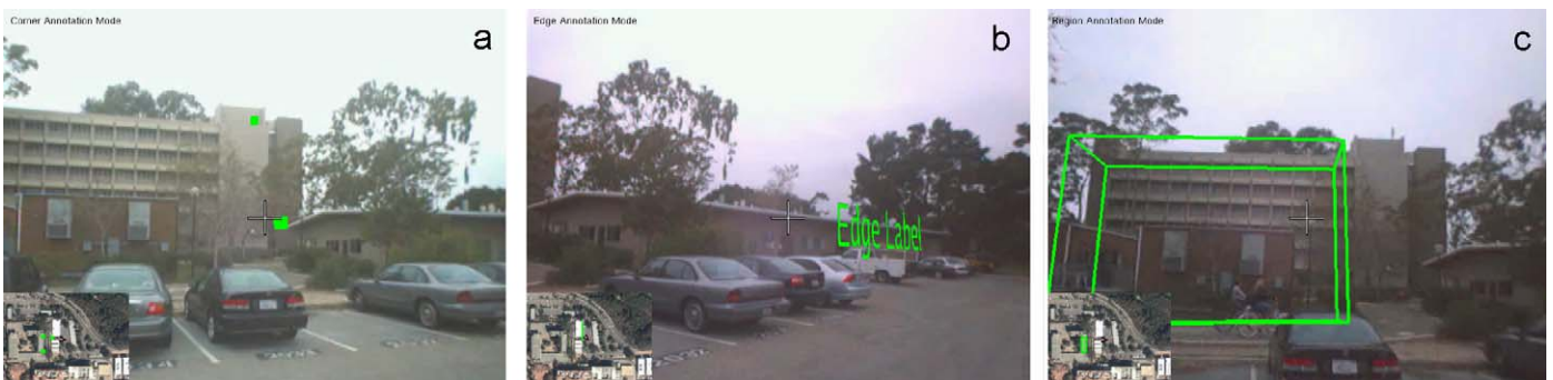
Fig. 7. Example annotations as seen by the user in first person view mode. Left to right: (a) corner annotations on the corners of two buildings are rendered as cubes. (b) An edge is annotated with a texture mapped onto the plane of the wall it denotes. (c) A region annotation is rendered as a wireframe bounding box. These renderings are not geared toward a particular application; rather, they are for illustrative purposes. Applications using these annotations would have visual representations tailored to their needs.
