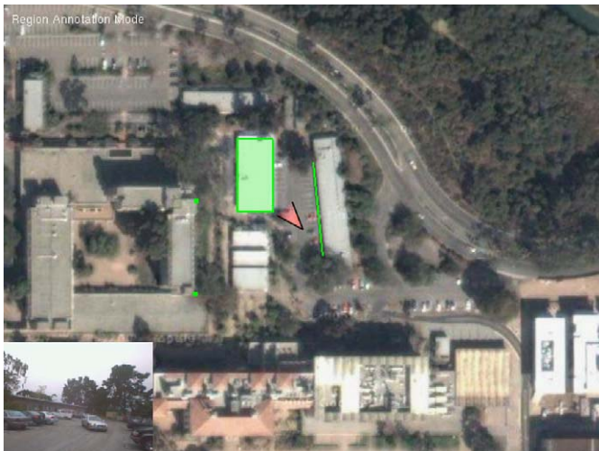
Fig. 6. The aerial photograph view from within the aerial photograph based annotation system. In the lower left corner, an insert of the video feed from the display mounted camera can be seen. The user's position and orientation are represented on the photograph with a small cone avatar. A small set of features have already been annotated—two corners (the green points), one edge (the green line), and one region (the transparent green rectangle). (For interpretation of color in this figure legend, the reader is referred to the web version of this article.)
