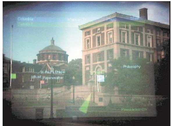
Fig. 7. Outdoor AR UI in accurate tracking mode (imaged through see-through head-worn display). Labels and features (interactive virtual flags denoting points of interest) are registered with the physical environment.
