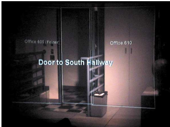
Fig. 5. AR UI in accurate tracking mode (imaged through see-through head-worn display). Labels and features (a wireframe lab model) are registered with the physical environment.
