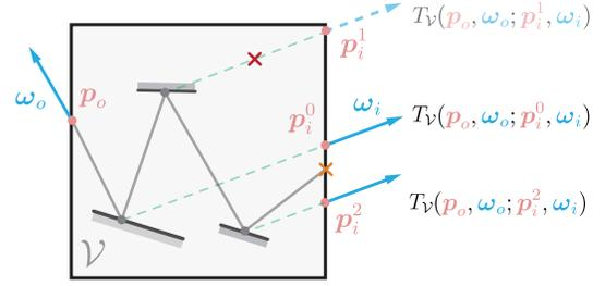
Fig. 14. To obtain reference samples for the appearance network, we can, in a single pass, aggregate multiple throughput samples for different exitant position  $\mathbf{p}_i$ . A red cross indicates a failed shadow test, while an orange cross indicates path termination at the voxel boundary.
