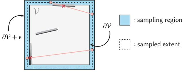
Fig. 13. Our sampling domain regularisation addresses floating point errors that can arise when surfaces are close to the original voxel boundary.
