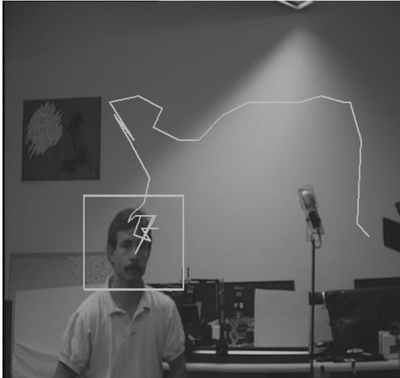
**Figure 5-3:** The head has been located — the image in the box is sent to the face recognition process. Also shown is the path of the head tracked over several previous frames. (The subject entered the scene from the right, walked over and sat down.)
