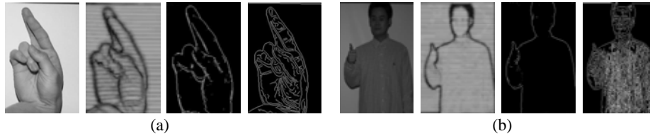
Fig. 8 (a) Detection of depth edges in the case of hand gestures for fingerspelling, (b) Detecting human body contours for gesture recognition, from left to right: white light image, Gabor amplitude map, depth edges and canny edges.
