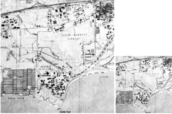
Figure 2. left A map image I_1 . right The thumbnail I_2 after applying the forward wavelet transform. left
