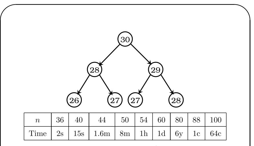
Time complexity of above method is  $\Omega(2^{n/2})$ . But it can be computed in O(n) time and constant space.
