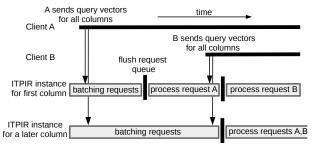
Figure 6—Batching at an object server in Popcorn. Requests to the initial column from two clients A,B are in separate batches as the processing cycle for this column is short. The requests to a later column (sent alongside the requests to the first) can be batched. This arrangement is inspired by Pyramid Broadcasting [105].
