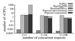
Figure 10—Per-request server-side resource use (log-scaled) of Popcorn and the baselines with varying concurrent requests *C*. If I/O is the bottleneck, there are idle CPU cycles and vice versa (§4.3). For Popcorn, we depict both the provisioned and consumed resources; for the baselines, we depict only the latter. We do not depict I/O usage for NoPriv as it is always zero (see text).
