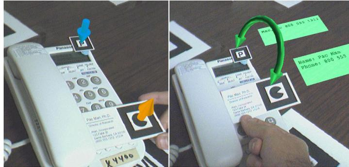
Figure 3: Application interaction. *left*: phone (data handler) and business card (data container). *right*: phone receives business card data, displaying and storing the name and phone number.
