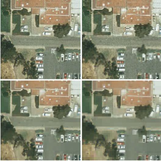
Figure 3: Comparison of 2D image compression, zoomed in to show detail. Clockwise from Top-Left: (a) Original  $16384^2$  image, uncompressed at 768MB. (b) Downsampled to  $4096^2$ , largest size supported by our graphics card, at 50MB, RMS error 0.65. Detail is uniformly lost everywhere. (c) Wavelet compressed to 138MB (ratio of 5.6), RMS error 0.027. High-frequency information remains. (d) Wavelet compressed to 42MB (ratio of 18.3), RMS error 0.046.
