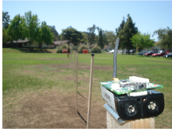
Figure 4: Static scenario: stick. The sender is located on the first stick, the receivers are positioned on the following sticks.
