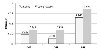
Fig. 2: Comparison showing power-efficiency of the poweraware scheduler with bars representing baseline (left) and power-aware (right) efficiency for three production traces (DS2, DS3, and DS5).
