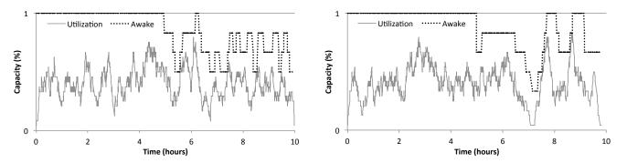
Fig. 1: Timeries showing synthetic exponential (left) and lognormal (right) workload trace with power-optimizing scheduler activated at the 5 hour mark. The x-axis depicts time in one hour intervals, and the y-axis shows the fraction of the number of cores occupied. The dotted line shows the fraction of cores that belong to nodes that are powered-up.
