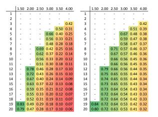
Fig. 5: Parameter-sweep predicts changes in power-efficiency with increasing node count (y-axis) and workload intensity (Lognormal arrival,  $\mu$  on x-axis,  $\sigma = 1.0$ ) at the baseline (left) and with power-aware scheduler (right).
