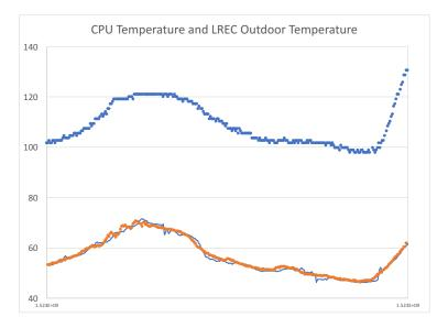
Figure 2: Time series trace of outdoor temperature, CPU temperature, and predicted outdoor temperature taken from LREC. The units of the y-axis are degrees Farenheit. The sensor generates a measurement every 5 minutes.
