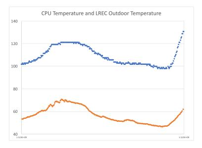
Figure 1: Time series trace of outdoor temperature and CPU temperature taken from LREC. The units of the y-axis are degrees Farenheit. The sensor generates a measurement every 5 minutes.
