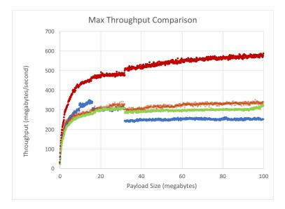
Figure 5: Comparison of maximum throughput rates as a function of payload size across edge and cloud platforms
