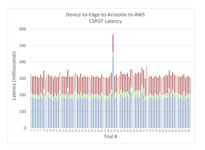
Figure 6: "Chain" replication from Raspberry Pi to edge cloud to Aristotle to AWS. 100 sepparate, backto-back trials (*x*-axis). The lowest section of each bar (blue) depicts Pi-to-edge latency, the second from the lowest (green) shows the edge-to-Aristotle latency, and the top part of each bar (red) shows Aristotle-to-AWS latency. The units are milliseconds.
