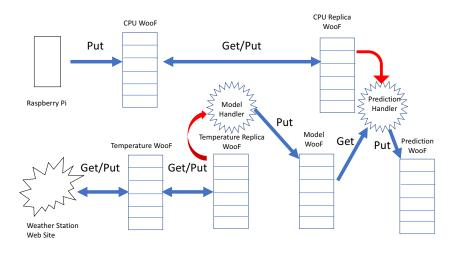
Figure 3: CSPOT Frost Prevention Application Structure
