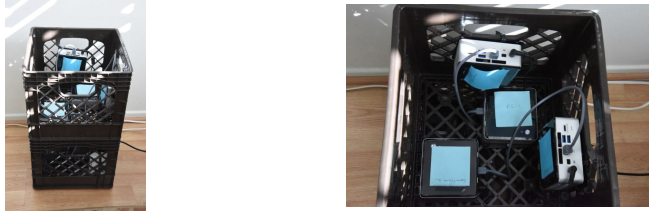
Figure 2: Prototype SMARTFARM appliance for on-farm deployment. Top half contains compute elements running SMARTFARM software stack. Bottom half contains network switch and uninterruptable power supply (UPS).
