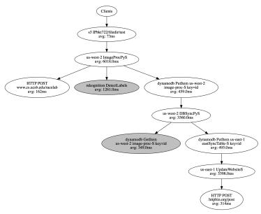
Fig. 3: *GammaRay* service graph for ImgProc [30]. *GammaRay* captures causal dependencies and performance through AWS services and across regions.
