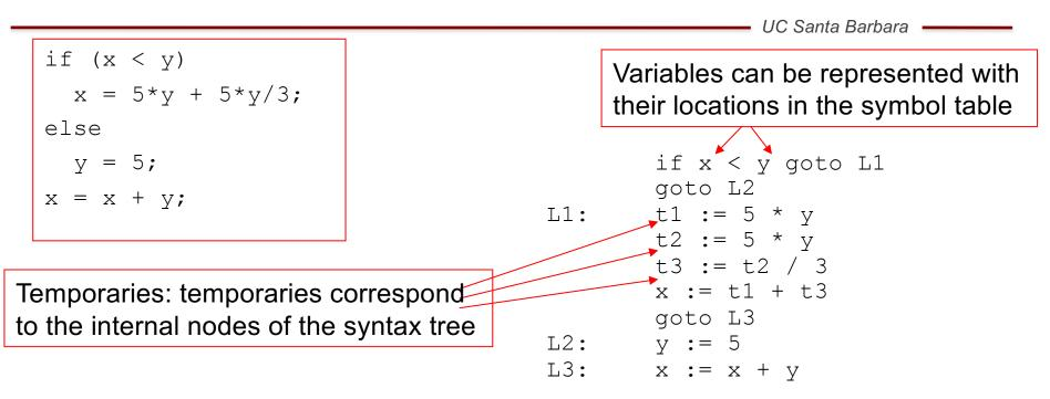
• Three-address code instructions can be represented as an array of quadruples: operation, argument1, argument2, result triples: operation, argument1, argument2 (each triple implicitly corresponds to a temporary)
