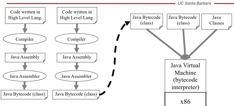
Here the compiler targets java bytecode (which is what we do in this class) and the bytecode is then run on top of the Java Virtual Machine (JVM). The JVM really just interprets (simulates) the bytecode like any scripting language. Because of this, any java program compiled to bytecode is portable to any machine that someone has already ported the JVM too. No need to recompile.
