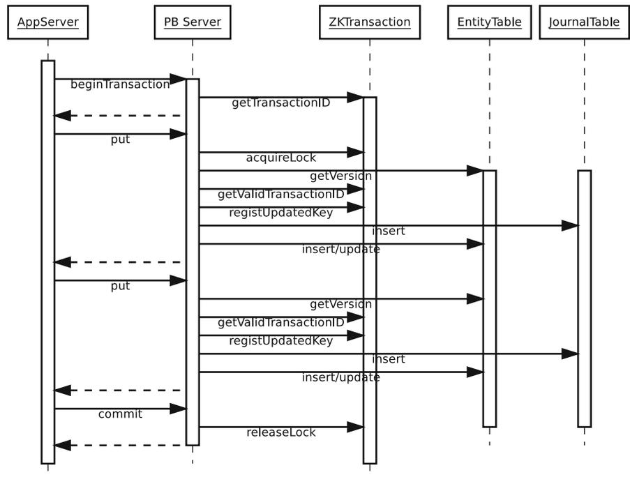
transaction starting where a transaction ID is attained; a *put* request then triggers the acquisition of a lock, version validation, key registration for rollback, and entity updates. The second *put* repeats the same steps sans lock acquisition. Lastly, the transaction is committed.
