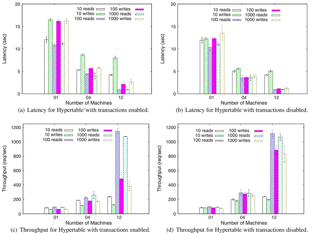
Fig. 6 Hypertable results as the number of machines increases
