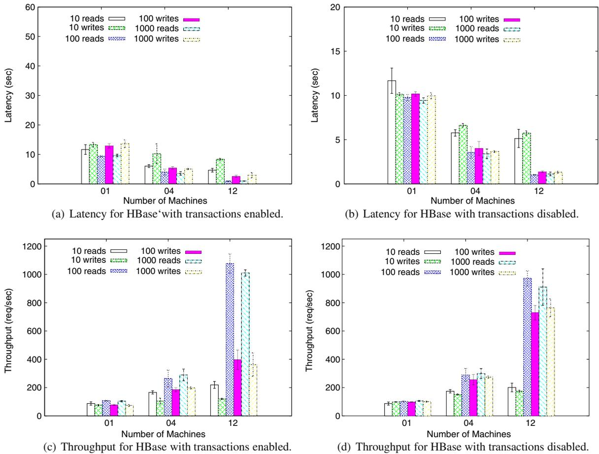
**Fig. 5** HBase results as the number of machines increases
