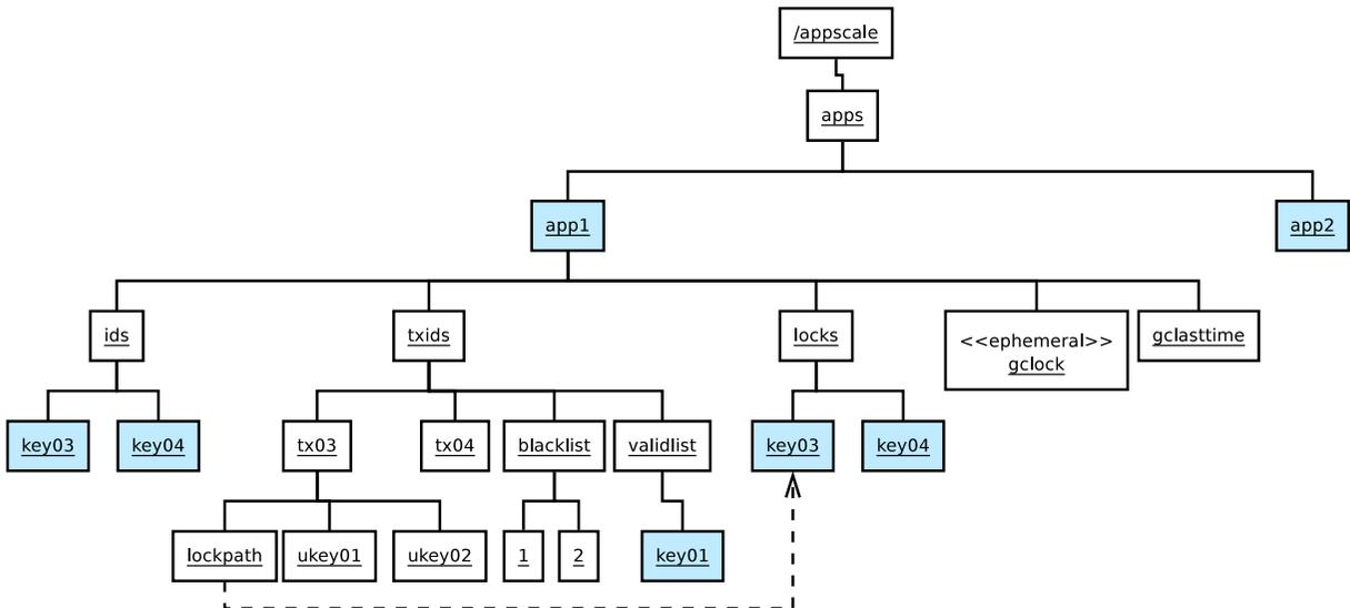
Fig. 3 Structure of transaction metadata in ZooKeeper nodes
