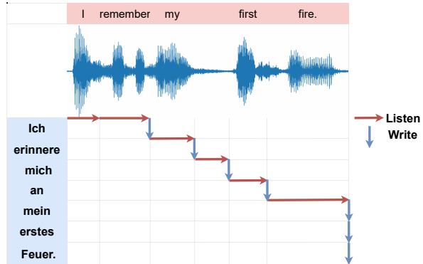
Figure 1: An illustration of streaming speech-to-text translation. ST models listen to the audio in source language, and generate tokens in target language.
