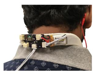
Figure 3: The second and final GVS prototype in the form of a small wearable device that sits on the user's neck, similar to behind-the-head earphones. The red wire connects the circuit to an electrode behind the user's ear. A similar wire connects to a second electrode behind the other ear. The white wires connect to EDA and HR sensors.
