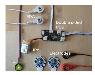
Figure 6: Our GVS device without the 3D printed housing. The image shows the EDA and HR sensors plugged into the PCB using the onboard connection ports.
