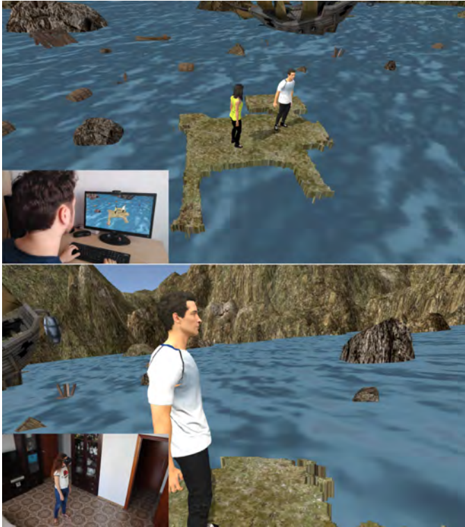
Fig. 12. Example of asymmetrical multiuser scenario. Male avatar user is connected through a computer, as shown in top image inset, while the female avatar user is connected using a Tango tablet worn as an HMD, as shown in the bottom image inset. The RE corresponds to 4a. In this case there is no need of a WA combination as only one RE is used.
